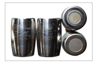
Fig. 35 Scoring on the Roller End Face
