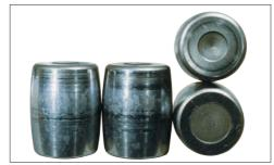
Convex rollers of Photo 2-1 Symptom: Round shaped peeling pattern occurs on the center of the rolling surfaces
