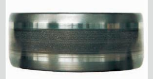
Part: Inner ring of a cylindrical roller bearing Symptom: Belt pattern of electrical erosion accompanied by pits on the raceway surface
