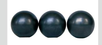
Part: Balls of a deep groove ball bearing Symptom: A dark color covering the entire ball surface
