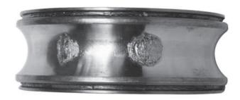
Fig. 4.1 Example of Flaking
