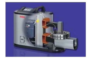
Fig. 5 Heating by bearing heater
