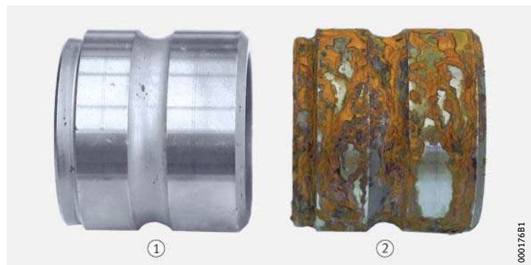
15 Coated and uncoated part after a salt spray test
